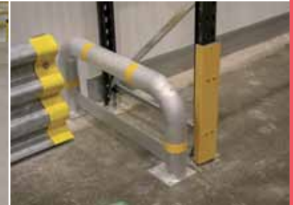
RACK END BARRIER
