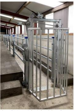
Above: Friction Lock Crush Gate & Front Gate
